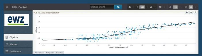
Analysis of the correlation between temperature and energy consumption ensures the correct functioning of thermal engineering system and the mapping of power consumption and load profiles for various properties.
