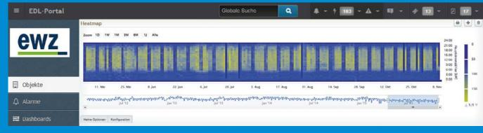
The heat map is especially useful for discerning consumption patterns and identifying any discrepancies
