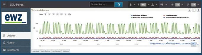
Monitoring and mapping of the power consumption and load profiles for various properties.
